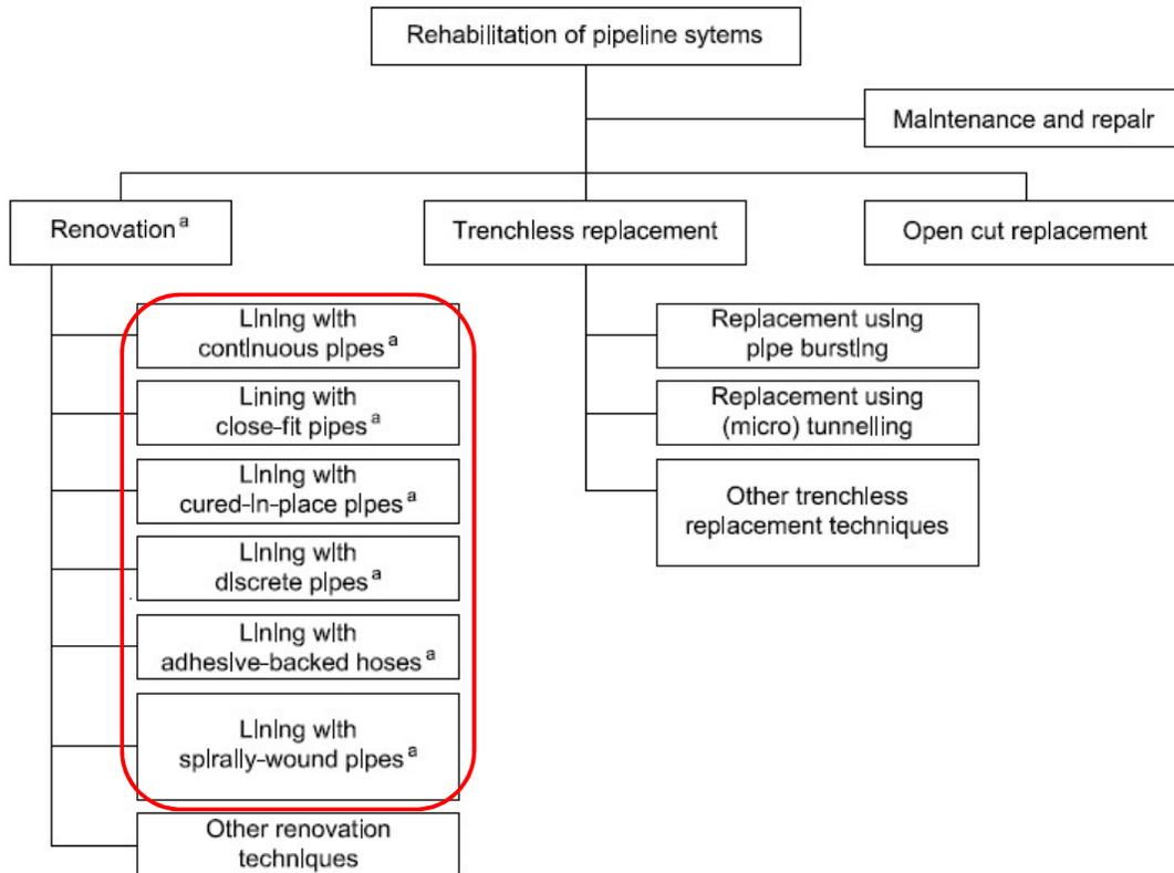
**Figure 1. The red box identifies the trenchless techniques that are covered in EN ISO 11295**
