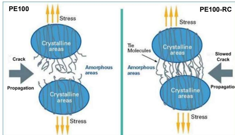
**Figure 3. The greater number and longer side branches of PE100-RC resist the initiation and growth of the crack through the pipe wall**
